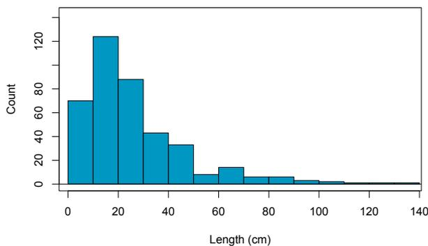
Fig. 4. Histogram of the synthetic dataset fracture lengths. Length  $\text{lognorm}(\text{meanlog} = 3.00, \text{sdlog} = 0.73)$ .
