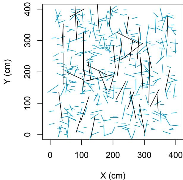
**Fig. 2.** Discrete Fracture Network graphical representation of the (synthetic) dataset. The 10% largest fractures are highlighted in black.
